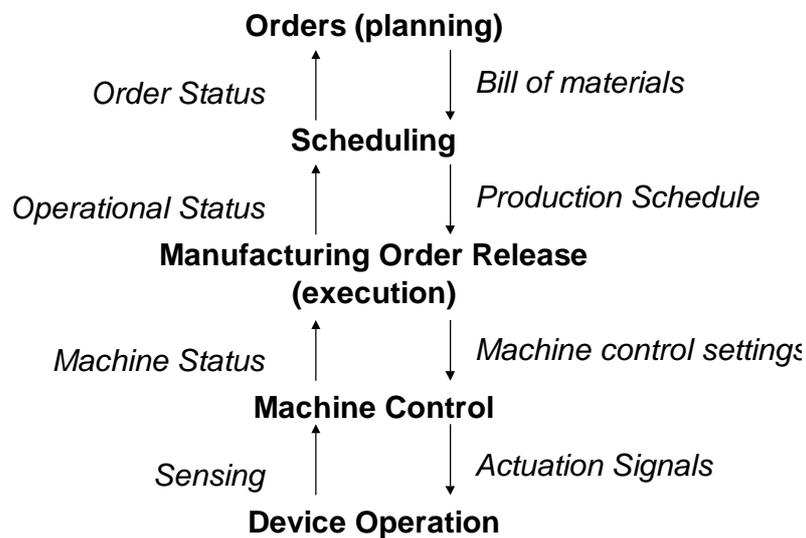
**Figure 5 Typical Manufacturing Control Hierarchy**
