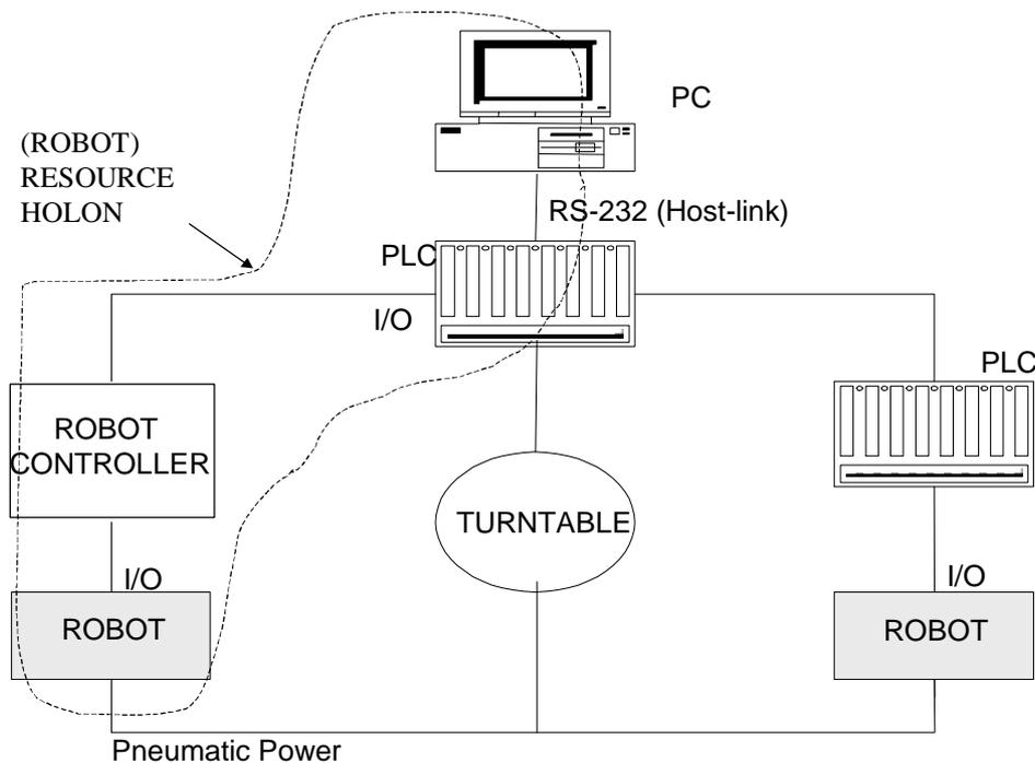
**Figure 9 Holonic Control Implemented in Conventional Infrastructure[81]**
