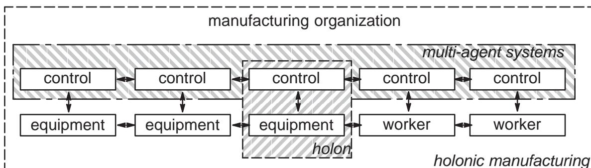
Figure 4: Views of HMS and MAS on manufacturing process.
